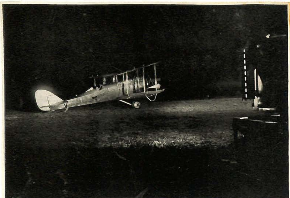
CAM 1 A NIGHT AIR MAIL PLANE ILLUMINATED BY A HALF-BILLION-CANDLEPOWER FLOODLIGHT AT HADLEY FIELD, NEW JERSEY Photograph Courtesy U. S. Post Office Department
