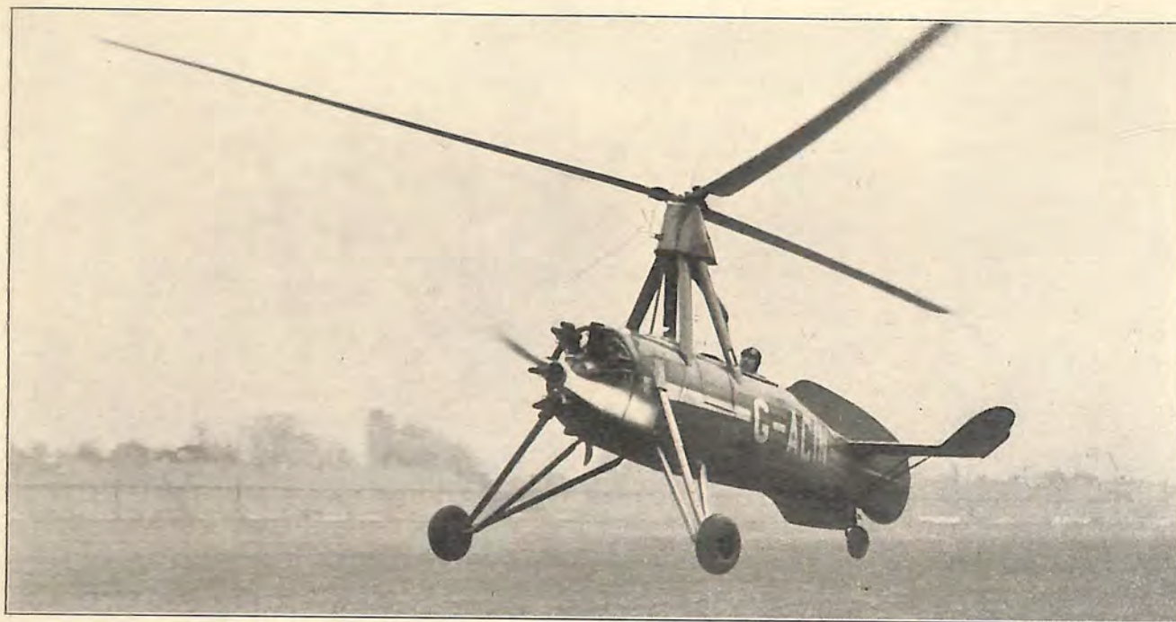
GETTING AWAY.—A test pilot taking-off in a C.30 Autogiro (140 h.p. Seven-cylinder Siddeley Genet Major)
