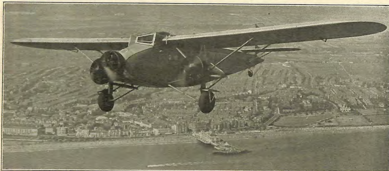
The Westland Wessex cabin monoplane (three Armstrong Siddeley Genet-Major engines), which is described on the previous page.—(“Aeroplane” photograph.)
