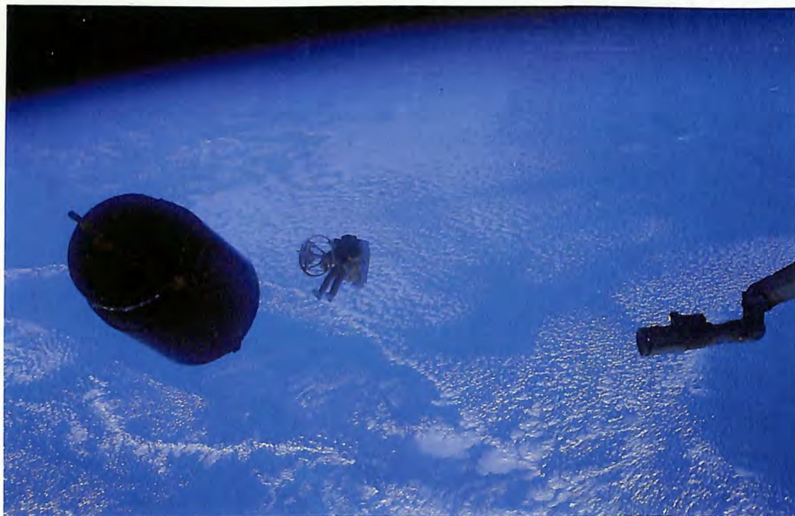
Dale Gardner, flying the MMU, makes a careful approach to Westar in this photograph taken from Discovery's flight deck windows. Mounted in front of Gardner is the stinger that will snare the satellite.
